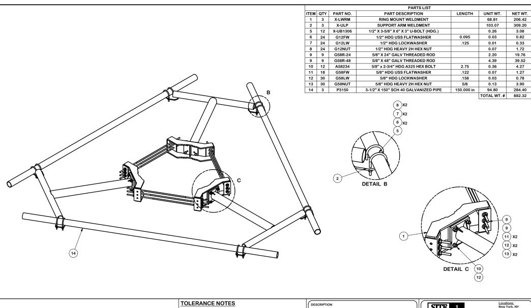
TOLERANCES ON DIMENSIONS, UNLESS OTHERWISE NOTED ARE: SAWED, SHEARED AND GAS CUT EDGES (\$ 0.030") ORILLED AND GAS CUT HOLES (\$ 0.030") - NO CONING OF HOLES LASER CUT EDGES AND HOLES (\$ 0.010") - NO CONING OF HOLES
